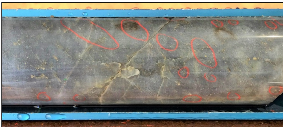
Photo 1: Typical silica-albite-sulphide Tura Lode mineralisation in BBDD1135 at 246.70m (assaying 184.64g/t Au). Multiple clusters of fine visible gold are circled in red. Core diameter is 47.60mm.
