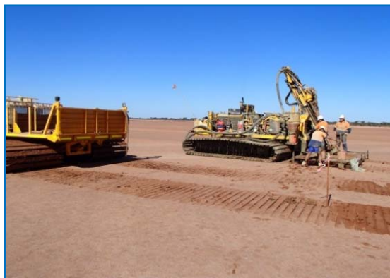
Photo 1: Aircore Drilling on Lake Roe Salt Lake
