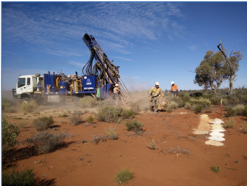
Photo 2: Aircore Drilling at Duketon North Project
