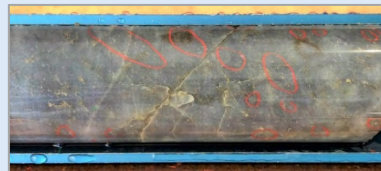
Typical silica-albite-sulphide Tura Lode mineralisation in BBRD1135 at 246.70m (assaying 184.64g/t Au); Multiple clusters of fine visible gold are circled in red; Core diameter is 47.60mm*
